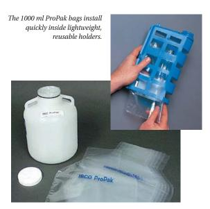
Our 2-gallon ProPak bags fit inside a rugged 2.5-gallon vented bottle. An O-ring holds the bag in place until the screw-on cap is installed.
