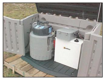
Challenges presented by the airport monitoring sites include the absence of telephone lines and AC power. These challenges were met by using cellular telephones for remote communication with the samplers, and a deep cycle battery and solar charger capable of powering the system with complete independence from utility lines.
