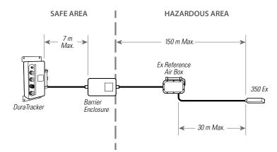
Figure 2-19350 Ex Area Velocity Sensor
