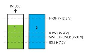
6. Bank 1 has reached the low SoC threshold (9.4 V). If battery bank 2 was not replaced (as shown in the previous instance), it is well below the low SoC. With both banks low, the DuraTracker unit returns to parallel mode.
