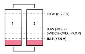
**Limp mode.** When both battery bank voltages drop below the 9.0 V (9.2 v in single batter bank) switch-over threshold, the DuraTracker unit will enter Limp mode, in which modem and Bluetooth functions are unavailable.
