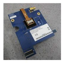
Figure 2-1 Non-Hazloc Modem
