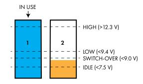
8. Or, possibly, neither battery is replaced, and both voltages drop below the switch-over threshold (9.0 V). The Dura-Tracker unit then enters Limp mode, as explained below.
