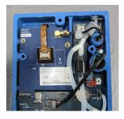
Figure 2-8 Connecting antenna cable
