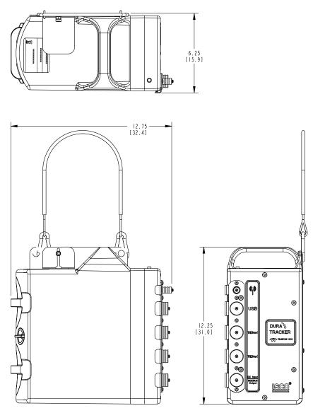
Figure 1-5 Specification Drawing, DuraTracker with Battery Box
