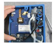
Figure 2-7 Plugging modem into circuit board
