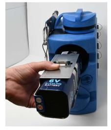
Figure 2-15 Installation of 6 volt lantern batteries
