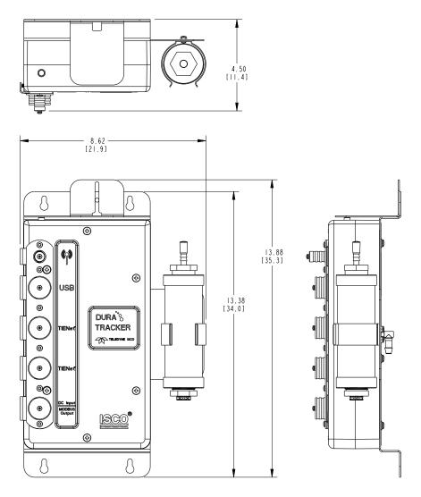
Figure 1-6 Specification Drawing, DuraTracker without Battery Box
