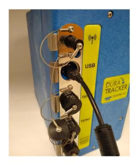
Figure 3-1 USB installation
