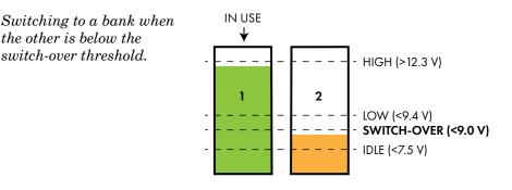
5. Battery bank 2 is replaced. But even though bank 2 has the highest SoC, the DuraTracker unit continues to run from bank 1. It will continue to do so until bank 1 reaches the switch-over threshold.
