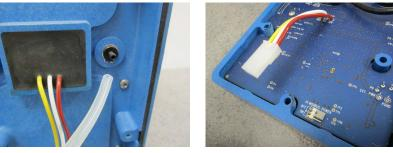
Figure 4-2 Disconnecting electrical connector and reference line
