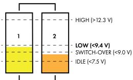
7. Possibly, battery bank 1 is replaced with a fresh bank that is above the low SoC threshold. In this case, the Dura-Tracker unit uses only bank 1 until it too falls below the switch-over threshold. (Compare to example 5, where *both* banks are still above that threshold.)
