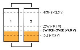
9. Eventually, both voltages drop could below the idle threshold (7.5 V). The DuraTracker unit then enters Idle mode, as explained below.
