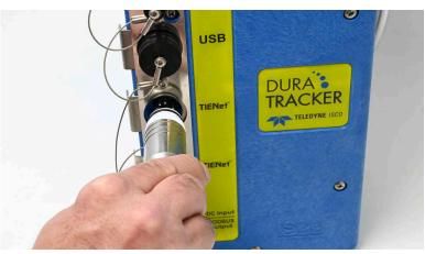
Figure 2-12 Connecting a TIENet sensor cable
