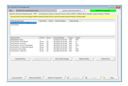
Figure 3-13 Data Storage Setup window
