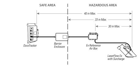
Figure 2-21360 LaserFlow Ex Sensor with Surcharge Sensor
