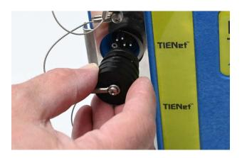
Figure 1-4 Capping the connector receptacle
