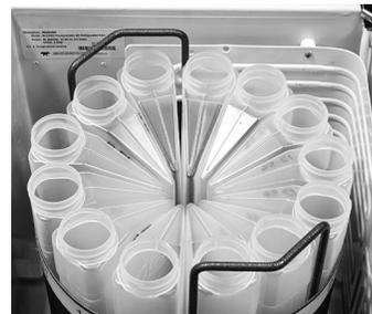
Figure 4—14-Bottle configuration completed
