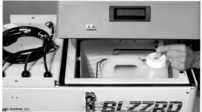
Figure 16—Insert the discharge tube when closing the compartment
