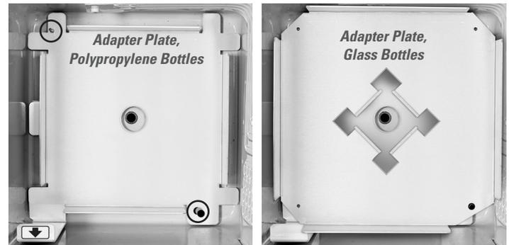
Figure 7—Adapter plates installed
